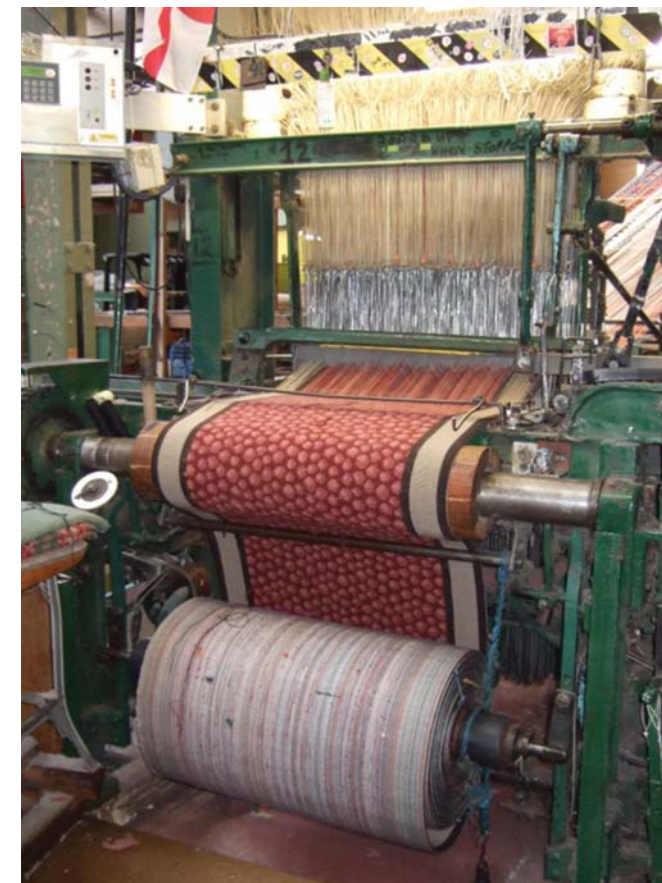
The Soane carpet in production on a Crossley loom. The pile is 100% wool and the colours were dyed in-house to a high intensity to achieve the depth of colour required
